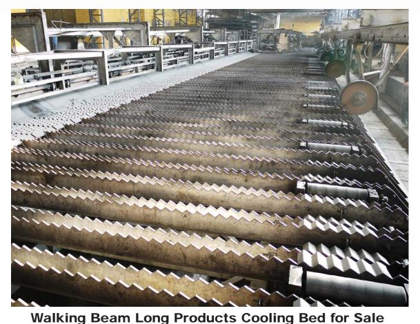
Age: 2004 Size: 30M Long x 5.4M Wide Capacity: 25MT per hour, 15-40mm dia rounds, flats Cycle Time: Approx 2 seconds Rake: 12mm thick with 90mm pitch x 35mm deep - 30/45deg Drive: Center mounted DC motor with heavy design lineshaft and eccentrics Controls: SCR Drive Cut to Length: Multiple Traveling Abrasive Saws
